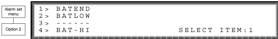
Figure 59: Battery parameters for alarm
